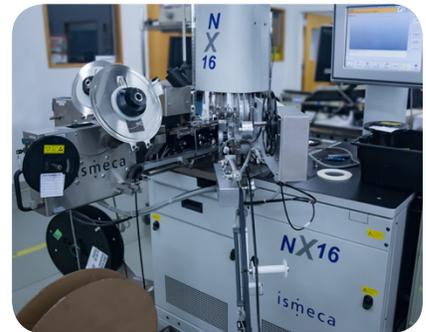
Devices can be custom screened for specific electrical parameters, and provided in accordance with customer-specified requirements.
