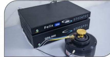
Particle Impact Noise Detection (PIND)
