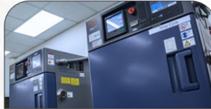
Temperature cycle testing
