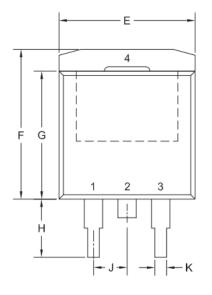
DIMENSIONS INCHES MILLIMETERS SYMBOL MIN MAX MIN MAX 0.189 4.14 4.80 0.163 В 0.045 0.055 1.14 1.40 С 0.000 0.00 0.25 0.010 D 0.012 0.028 0.30 0.70 Ε 0.386 0.415 9.80 10.55 F 0.378 0.417 9.60 10.60 G 0.335 0.358 8.50 9.10 0.188 0.236 4.78 6.00 Н 0.093 0.108 2.35 2.75 J 0.035 0.030 0.75 0.90
