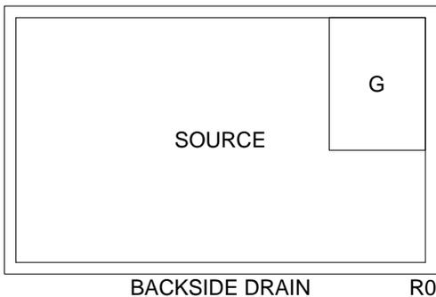
**Figure 2: CP406 Chip Geometry**
