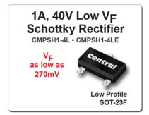
Hauppauge, NY USA – January 21, 2009 – Central Semiconductor Corp. announces the release of the CMPSH1-4L and CMPSH1-4LE Low  $V_F$  Schottky rectifiers with superior low  $V_F$  characteristics and packaged in the SOT-23F surface mount case. The CMPSH1-4L features a low forward voltage drop of 270mV @ 100mA, and 390mV @ 1.0A, while the enhanced version CMLPSH1-4LE, features low leakage currents of 200μA @ 5.0 Volts and 900μA @ 40 Volts.
