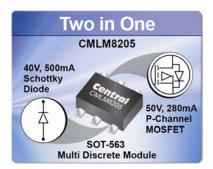
Hauppauge, NY USA – February 25, 2010 – Central Semiconductor Corp. announces the release of the CMLM8205 Multi Discrete Module in the SOT-563 surface mount package. This device features a 50V, 280mA P-channel enhancement mode MOSFET and an isolated 40V, 500mA low V<sub>F</sub> Schottky diode. The MOSFET has a minimum gate threshold of 1.0V and the Schottky diode has a low forward voltage drop of 0.35V at 100mA.
