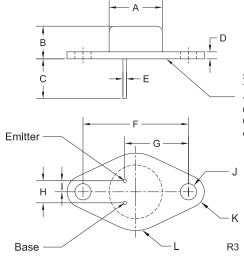
Seating Plane: The seating plane must be within 0.001" concave to 0.004" convex within 0.600" diameter from the center of the device.
